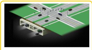
Cut and cover tunnel below rebuilt Huron Church Road/Highway 3 Corridor.
